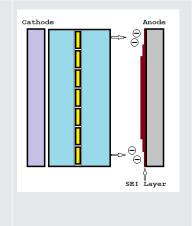
The maximum rate of intercalation of lithium ions into the anode decreases as the temperature decreases. This means that charge rates must be decreased to avoid excessive SEI build up. This can lead to lithium plating that can lead to a thermal runway condition.
