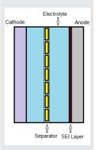
During discharge, lithium ions flow from the carbon layers in the anode to the oxide layers in the cathode.
